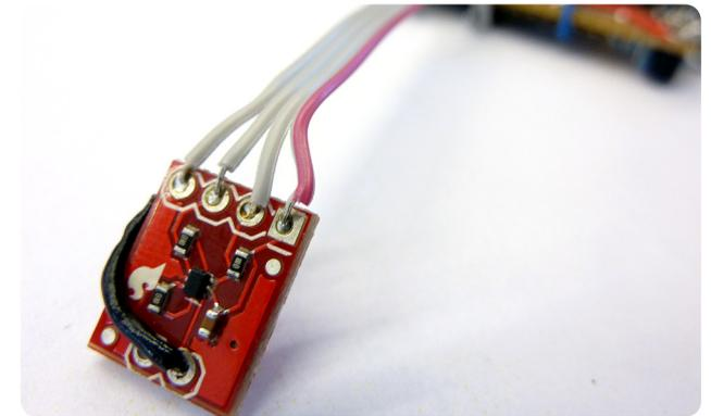
Close-Up of the TMP102 sensor temperature sensor
