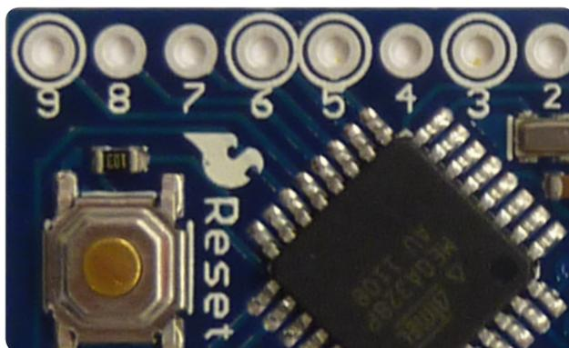
An Arduino Pro Mini micro controller
