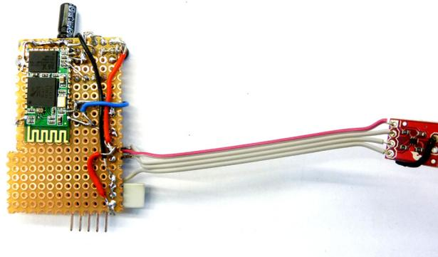
Sensor module with temperature sensor connected
