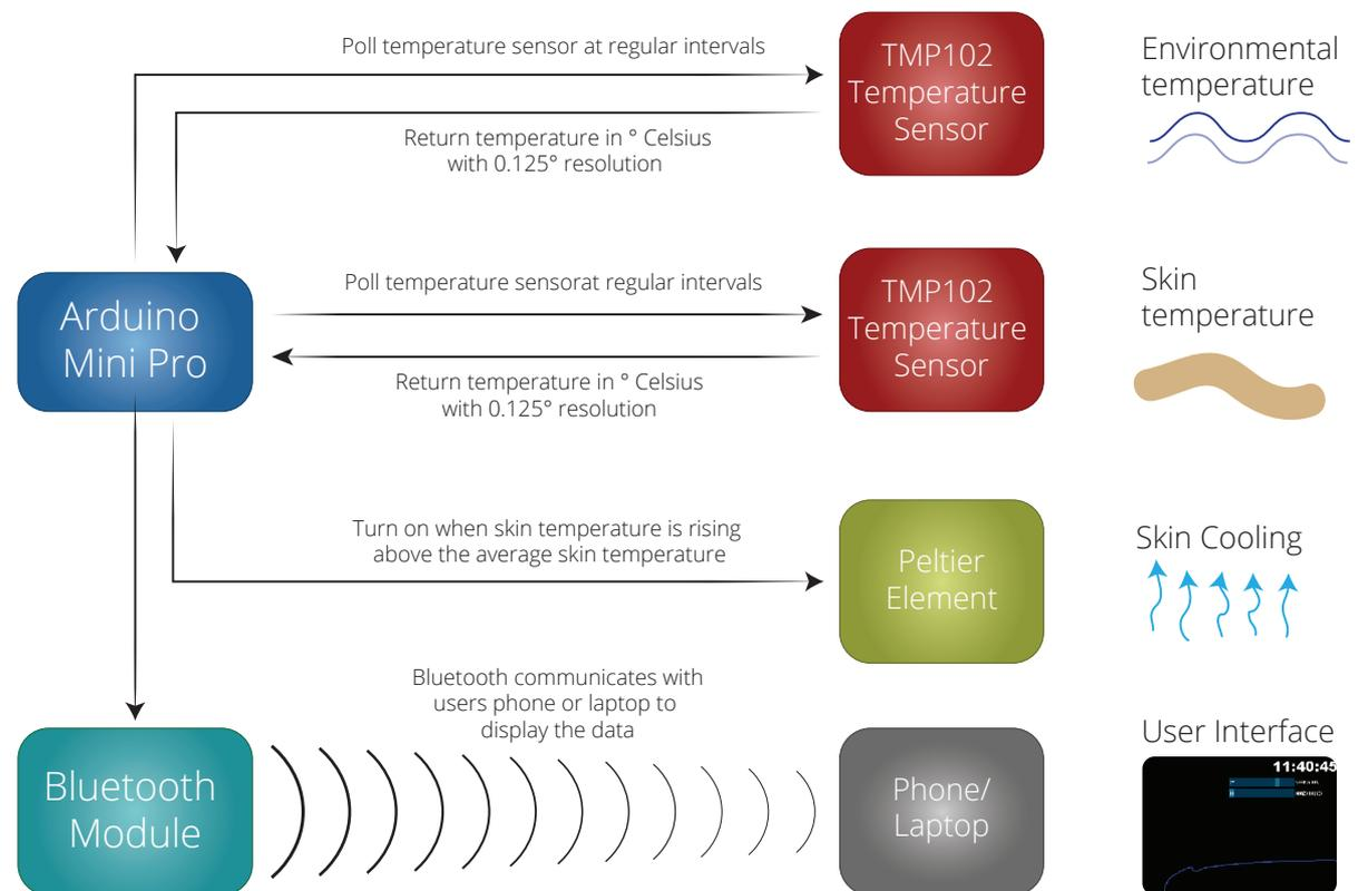
A visualisation of how the device would behave. The top two graphs do not represent actual measurements, but provide an example graph to demonstrate the device's workings. Real sensory data is used in the "Data Analysis" chapter.
