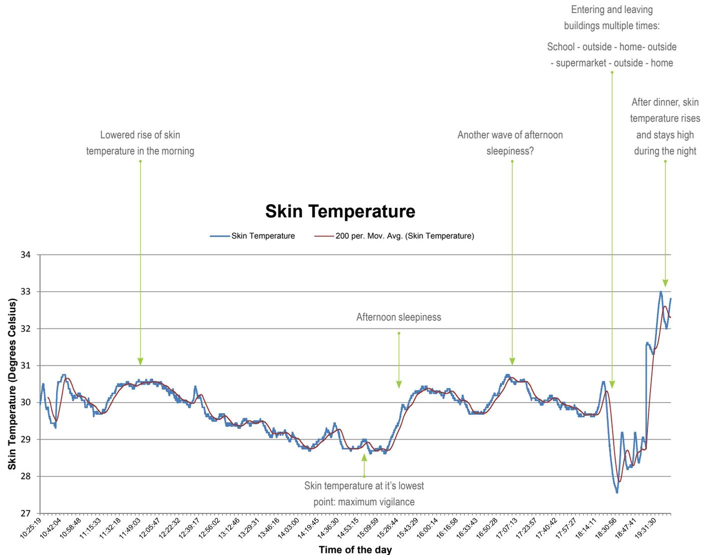
This graph shows measurements done with the prototype during a whole day. The blue line shows the measurements, while the red line shows the average based on 200 samples. It shows temperature fluctuations with different amplitudes during different times of the day. Some of these can be accounted to external influences, others can be a sign of vigilance drops.
