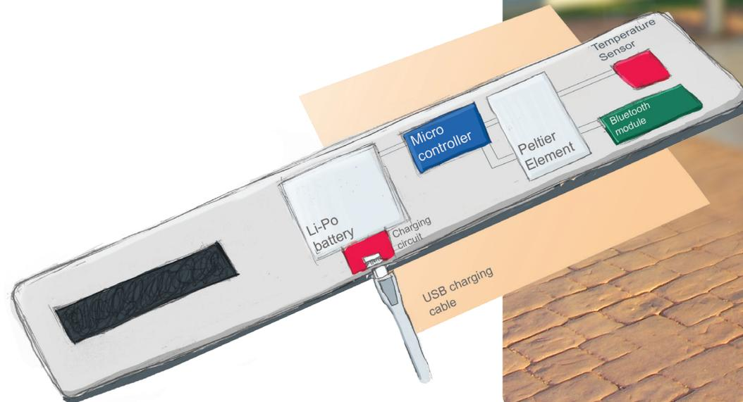
The different components, all integrated into the fabric wristband
