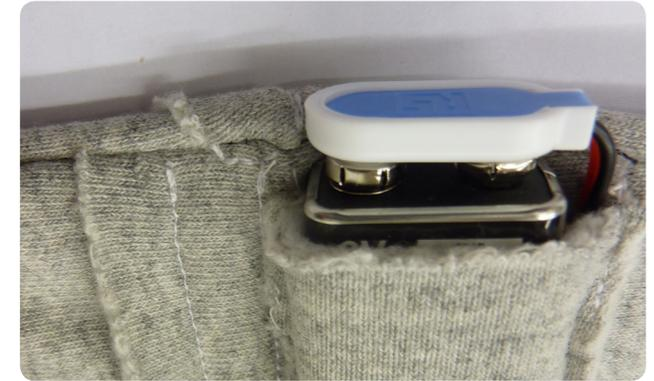
A 9V battery supplies power to the wristband
