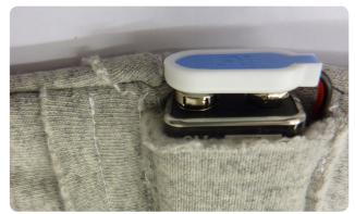
A 9V battery supplies power to the wristband
